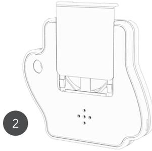
Apply pressure to slide the door up to unlock the back two tabs.
