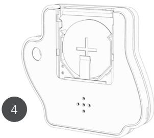
Locate the CR2032 battery. Notice the positive sign is on the top of the battery.
