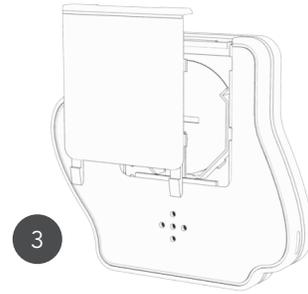
Once its loose, lift the door straight out of the back.
