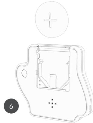
Pull the CR2032 up out of the battery contact.
